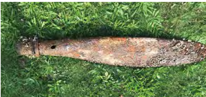
Propeller blade from Lt. Moody's Airacobra with bullet damage. Photograph by Wayne R. Lusardi, 2022.
